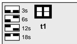
DIP switch pack **t1** determines the circuit breaker’s response time to an overload condition. Response times of three seconds, six seconds, twelve seconds, and eighteen seconds may be selected as shown in to the left. The **t1** DIP switches are factory set for a response time of eighteen seconds. POWERVAR recommends that these settings not be changed without first consulting POWERVAR Technical Support.
