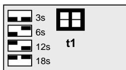
DIP switch pack **t1** determines the circuit breaker's response time to an overload condition. Response times of three seconds, six seconds, twelve seconds, and eighteen seconds may be selected as shown in Figure C to the right. The **t1** DIP switches are factory set for a response time of eighteen seconds. POWERVAR recommends that these settings not be changed without first consulting POWERVAR Technical Support.
